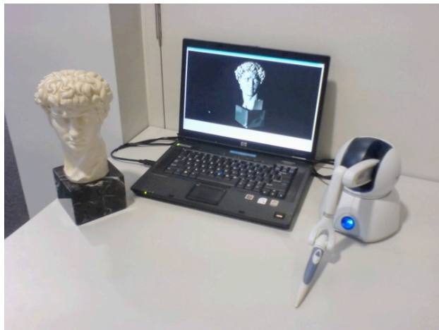
Figure 3: Physical and virtual sculpture with haptic device
