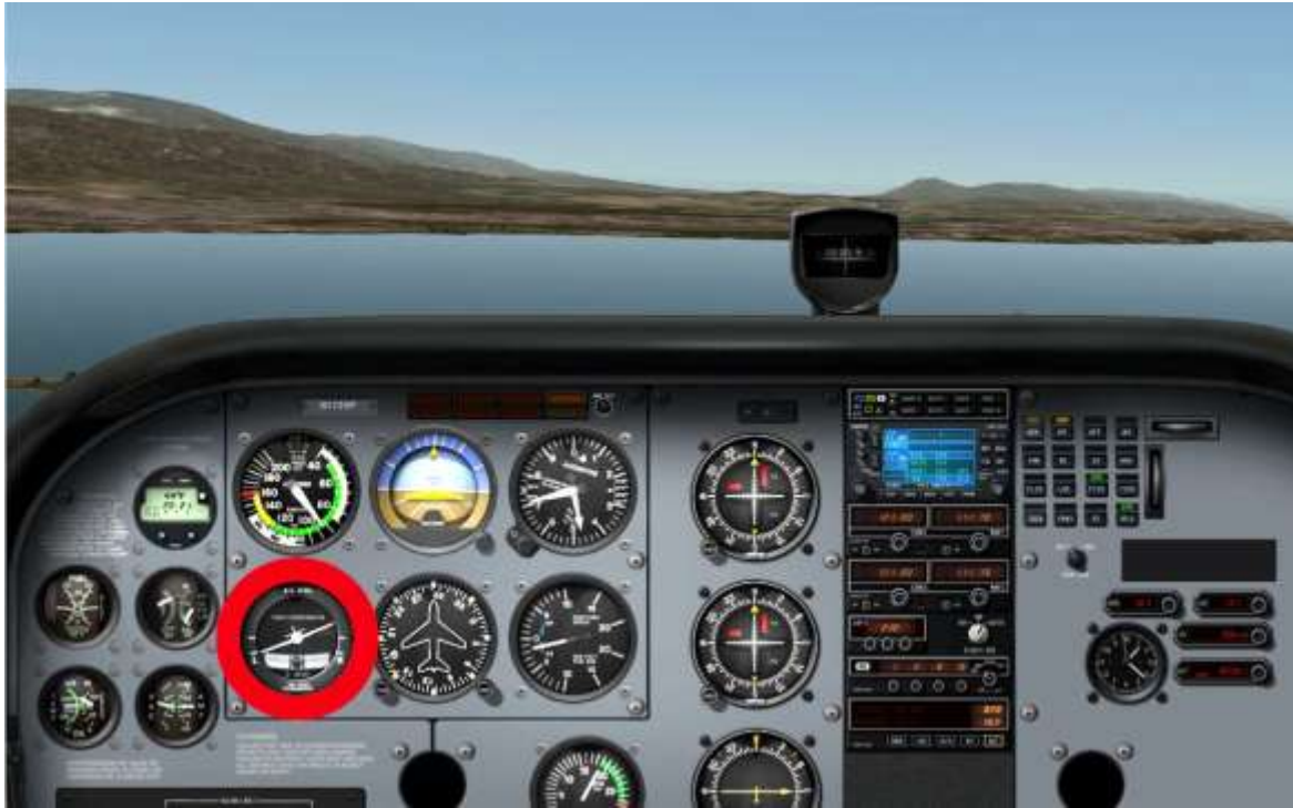
Figure 2: Example of a screenshot from the IFV task showing the aircraft flying straight and level. In this example, the Turn Coordinator (highlighted in red) has failed indicating a left turn while the remaining instruments suggest straight and level flight.
